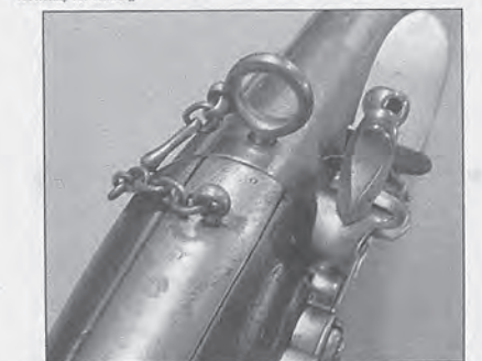
Figure 6- This view of the trigger guard shows where the pin penetrates (just in front of the large-headed screw). It has an eccentric end which enables the flat spring safety to move laterally when the pin is twisted.
